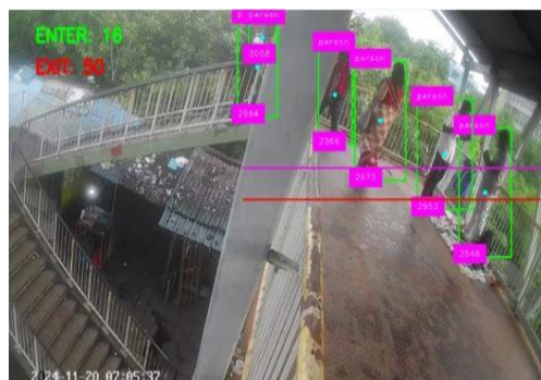
Figure 1. Using an AI Model Counting the Entry and Exit Passengers
