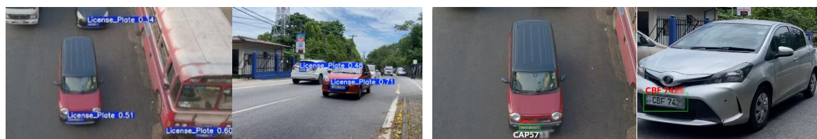
Figure 10: Output of NP Detection & recognition from Pedestrian Flyover and Ground Level, respectively
