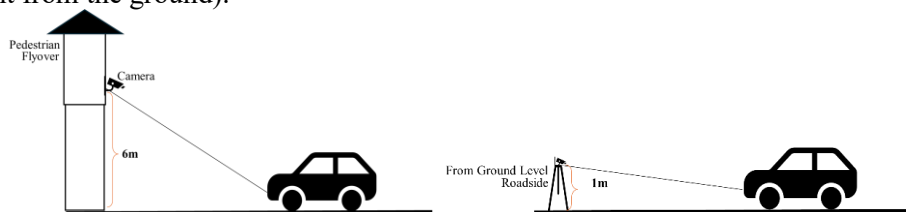
Figure 8: Side view of Camera position and Angle from pedestrian Flyover & Ground Level
