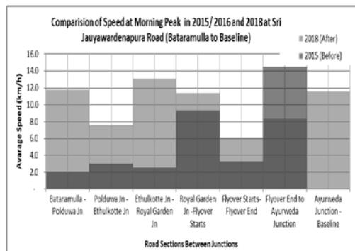
**Figure 4: Comparison of Speed at Main Rd**
